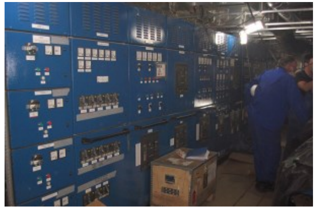
Main switchboard in the Engine room.
