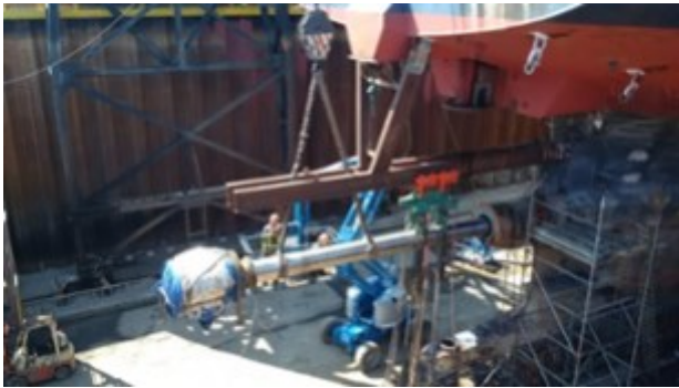
Algoma Spirit - tail shaft installation (L) and rudder stock / nozzle palm line boring (R).
