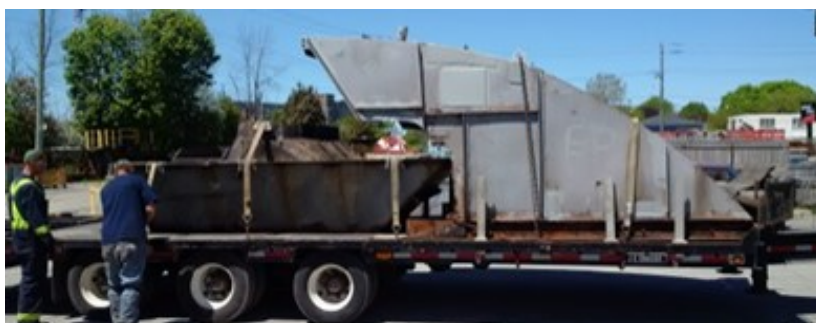
Algoma Enterprise - boom repairs underway (L) and boom hood deflector repaired and ready to be returned (R).
