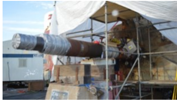
Algoma Spirit - tail shaft installation (L) and rudder stock / nozzle palm line boring (R).
