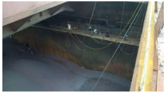
Algowood Longitudinal Bulkhead repairs with a storage load of Iron Ore.
