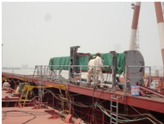
Accommodation ladder installed on DVS.
