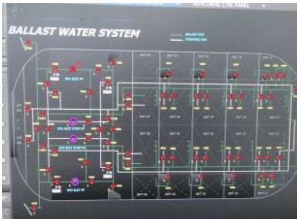
Ballast system control and mimic diagram.
