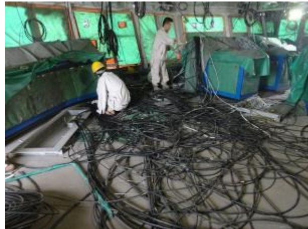
Wheelhouse consoles and wiring in progress.
