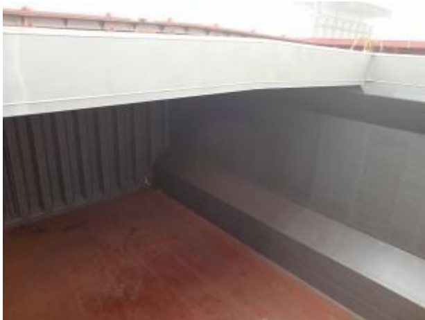
Cargohold – Note the clean lines and lack of arch webs.
