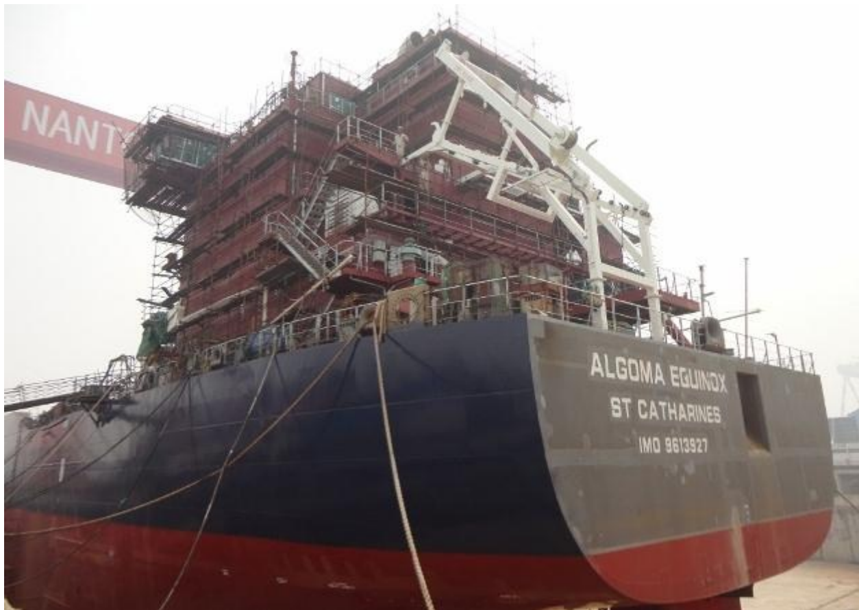
Aft view of the Algoma Equinox during installation of freefall lifeboat davit.
