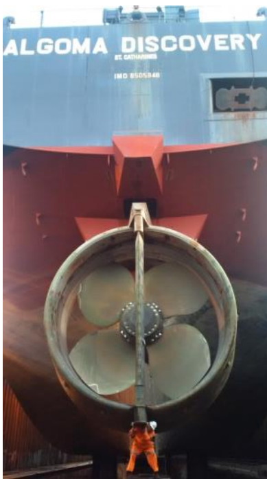
Repaired Kort nozzle.
