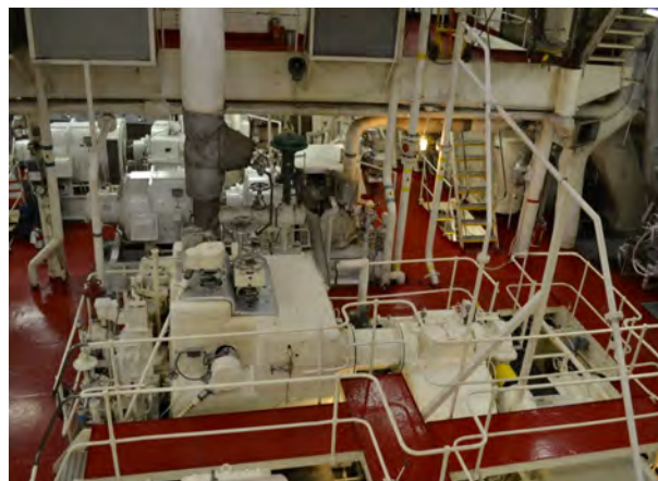
Side view of engine room machinery deck including main turbine and generator sets.
