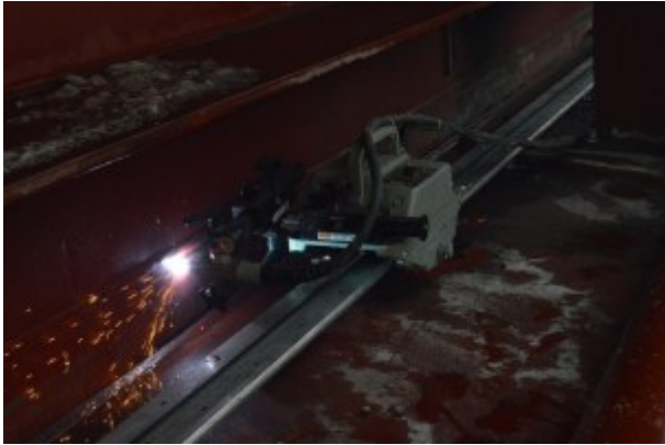
Main Cut Line in progress using automated drive Plasma Equipment on the Algoma Equinox .
