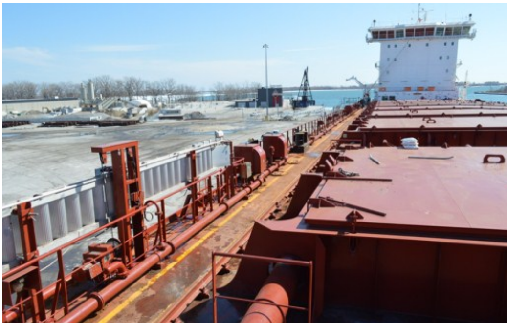
Outfitting Components installed. Midship Gangways relocated and secured on the Algoma Equinox .
