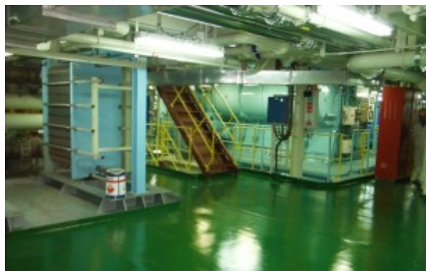
Central coolers, main engine in background on the Algoma Harvester.
