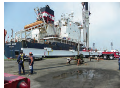
Above: Preparing to re-install the refurbished Gantry Crane on the Algoma Spirit .
