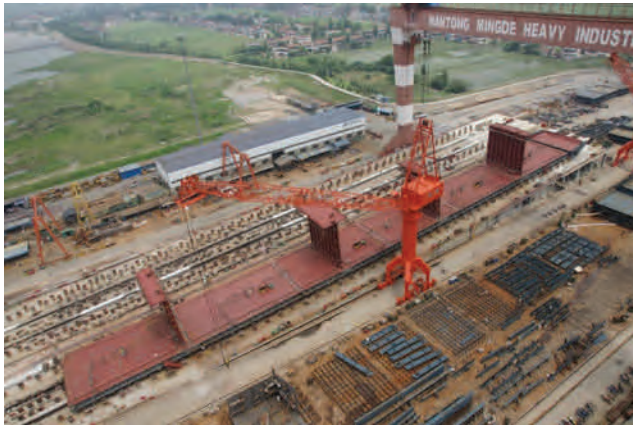
Double Bottom blocks with corrugated bulkheads
