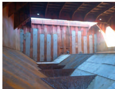
Above: Screen Bulkhead Repairs on the Algomarine in Port Colborne.
