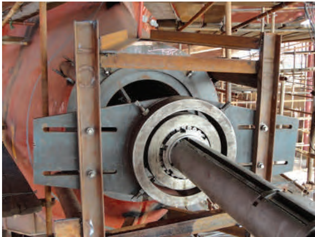
Stern tube machining prior to bearing installation
