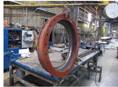
Above: Port Colborne Fairlead repairs
