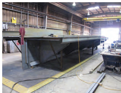
Above: Fabricating a Deck Arch to be installed on the John B Aird this winter.
