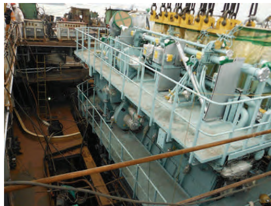
Main engine (Wartsila 5RT Flex 50) being lifted in to place on MD149 (December 3rd). The launching is expected to take place on December 18th.
