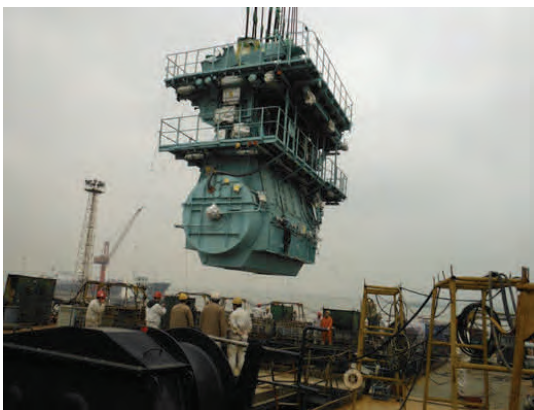
Main engine (Wartsila 5RT Flex 50) being lifted in to place on MD149 (December 3rd). The launching is expected to take place on December 18th.
