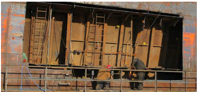
While berthed in Hamilton, ON, three sections of side shell plating on the Algosoo were repaired. Also, all the hatch covers for this vessel were removed and sealing channels were repaired and a new sealing rubber was installed.
