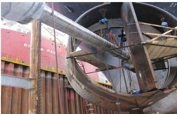
Tail Shaft inspection and repair on the Algorail.
