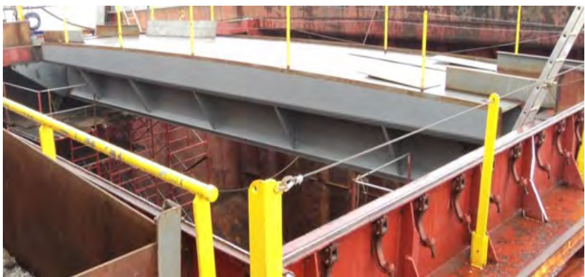
The Algomarine , berthed in Owen Sound, ON, received a new double deck arch between the #1 and the #2 hatch and a single deck arch between the #7 and the #8 hatch. These arches were fabricated in the shop and shipped up to Owen Sound.
